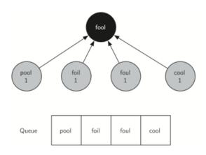
Starting from FOOL we take all nodes that are adjacent to FOOL and add them to the queue. The adjacent nodes include POOL, FOIL, FOUL, and COOL. Each of these nodes are new nodes to expand.
