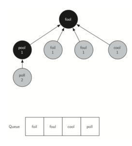
In the next step bfs removes the next node (**POOL**) from the front of the queue and repeats the process for all of its adjacent nodes.
