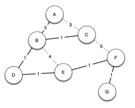
In this example A forwards the message to B. B forwards the message to D and C. D forwards the message to E, which forwards it to F, which forwards it to G. No router sees more than one copy of any message, and all the listeners that are interested see a copy of the message.
