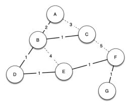
Below shows a simplified version of the broadcast graph and highlights the edges that form a minimum spanning tree for the graph.
